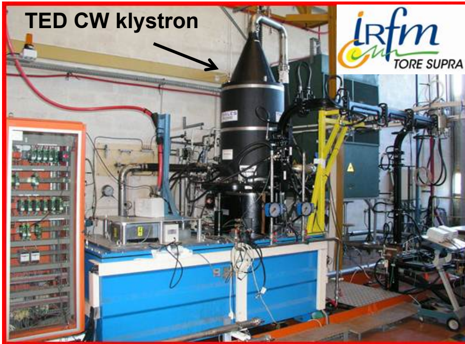
Test stand for 3.7 GHz klystrons at CEA-IRFM
